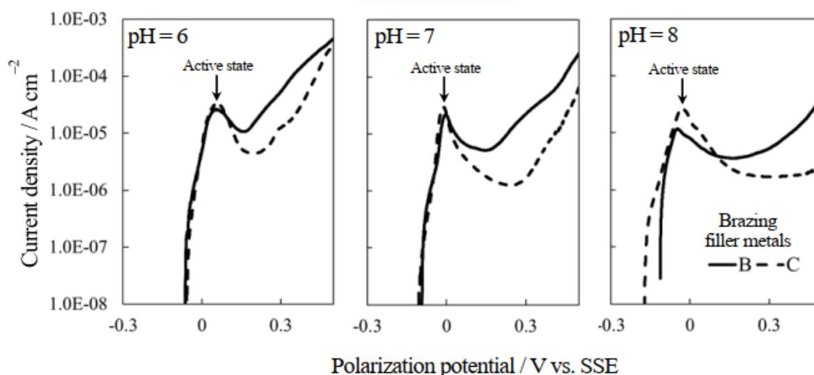
Fig. 3 Anodic polarization curves of the brazing filler metals of B and C at pH = 6, 7 and 8.
