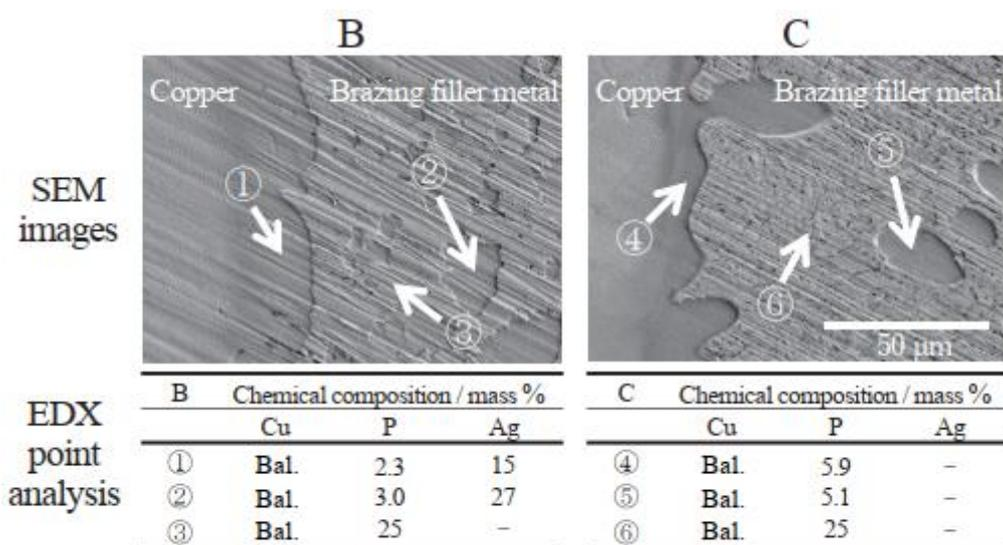
Fig. 1 SEM images of test materials and results of composition analysis by EDX point analysis at several points.
