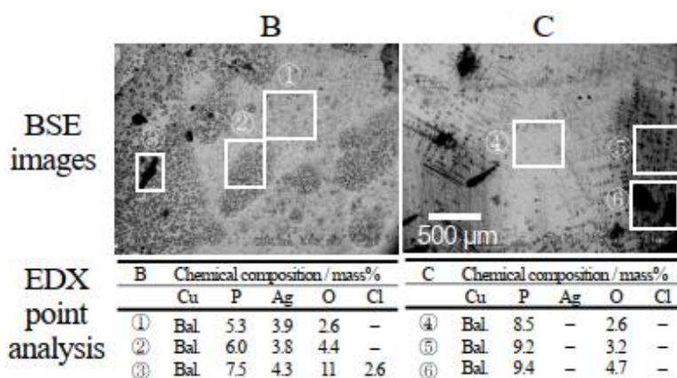
Fig. 5 BSE images of sample surface after anodic polarization measurement and results of composition analysis by EDX analysis at several regions of B and C at pH = 6.
